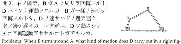
Problem2. When B turns around A, what kind of motion does D carry out in a right figure? When B turns with a same speed, which side is the speed of D fast or late? In addition, can you let move D adversely, and B do rotary motion?
