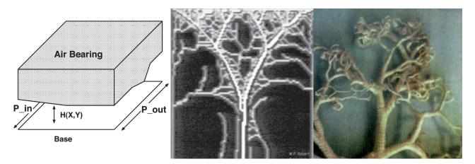
**Figure 3**—The geometry of an air-bearing is shown on the left. In this diagram, air flows under the bearing from left to right driven by a pressure drop. The computationally optimized surface of a static air bearing from the Mathematical Problems in Industry Workshop 2001 is displayed in the center. On the right, the circulatory system of a basket starfish, one of many examples of branching processes in the natural world.
