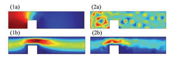
**Figure 1.**—Distribution of pressure (a) and norm of the velocity field (b) for two different simulations (I & 2) of the same situation
