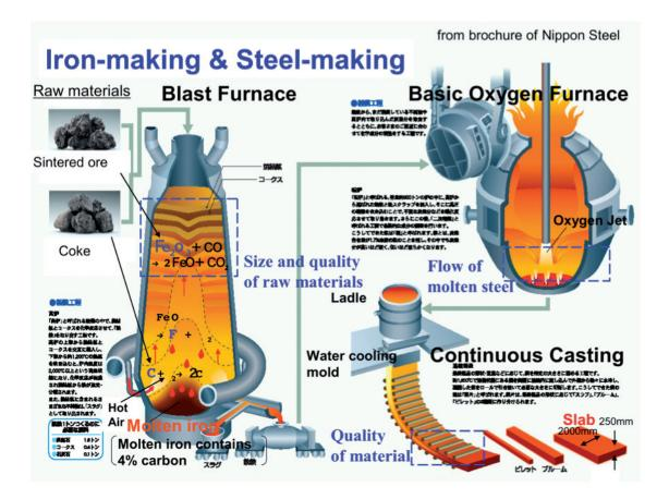
**Figure 4**—Example of inhomogeneous media in iron making and steel making process
