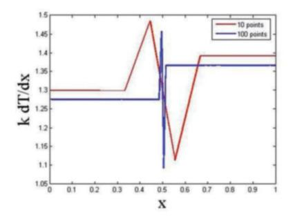
Figure 2.—Effect of grid refinement on the simulated flux
