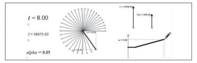
**Figure 2**—Modellus animation of the rotational motion of a wind turbine. The bar stroboscopic effect shows the acceleration due to the net applied torque.
